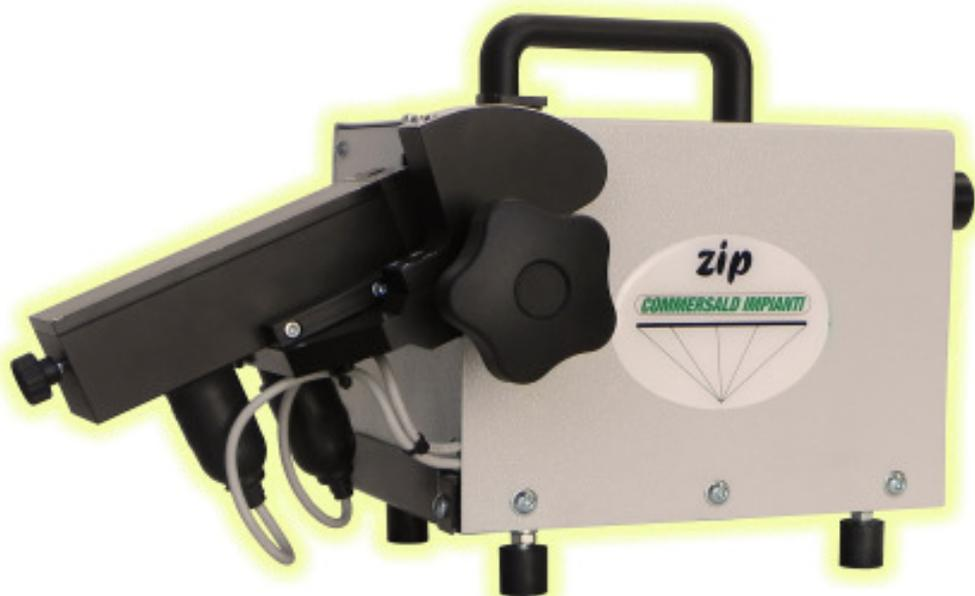
The standard version is used for electrodes from diameter **1,6 mm to 6,0 mm**, with the possibility to arrive till 12,00 mm using a special front panel. Every electrode is inserted into one hole, whatever diameter it has, because the machine has an **automatic adjustment system**.
